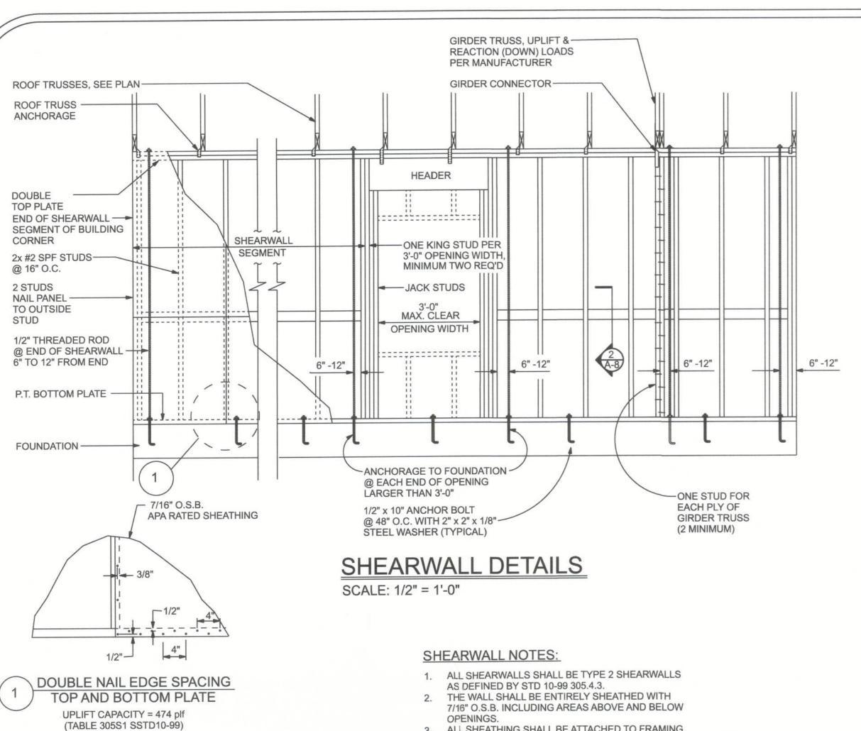
3. ALL SHEATHING SHALL BE ATTACHED TO FRAMING ALONG ALL FOUR EDGES WITH JOINTS FOR ADJACENT PANELS OCCURING OVER COMMON FRAMING MEMBERS OR ALONG BLOCKING.
