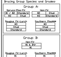
1x4 Braces shall be SRB (Stress-Rated Board) \*\*For 1x4 So. Pine use only Industrial 55 or Industrial 45 Stress-Rated Boards, Group B values may be used with these grades.
