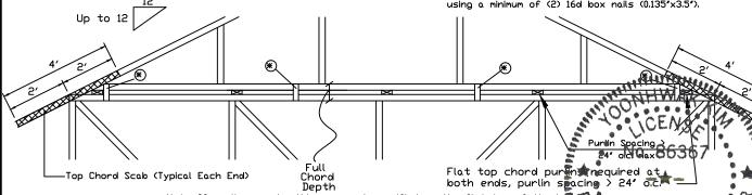
Note: If purlins or sheathing are not specified on the flat top of the bose 0 truss, purlins must be installed at 24" o.c. max. and use Detail A.
