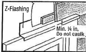
Figure 8 Ground to Siding
