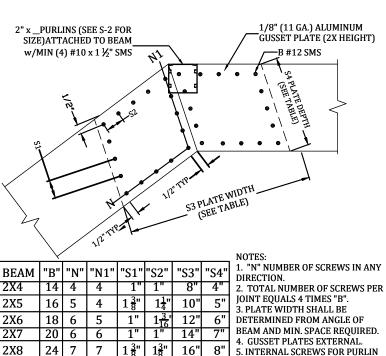
4. GUSSET PLATES EXTERNAL. 8" 5. INTERNAL SCREWS FOR PURLIN CONNECTION MAY BE INCLUDED IN 9' TOTAL NUMBER OF SCREWS. 9" 6. GABLE SPLICE WILL HAVE THE SAME PATTERN. 20" 10"
