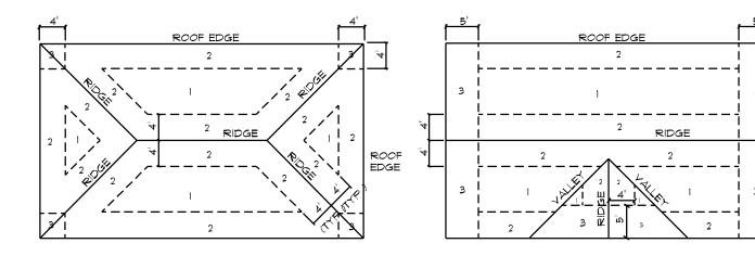
ROOF SHEATHING NAILING ZONES (HIP ROOF)
