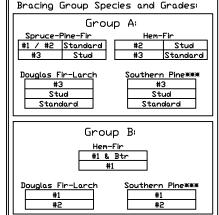
1x4 Braces shall be SRB (Stress-Rated Board).
