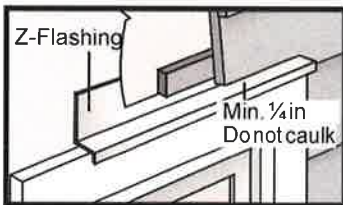
Figure 11 Ground to Siding
