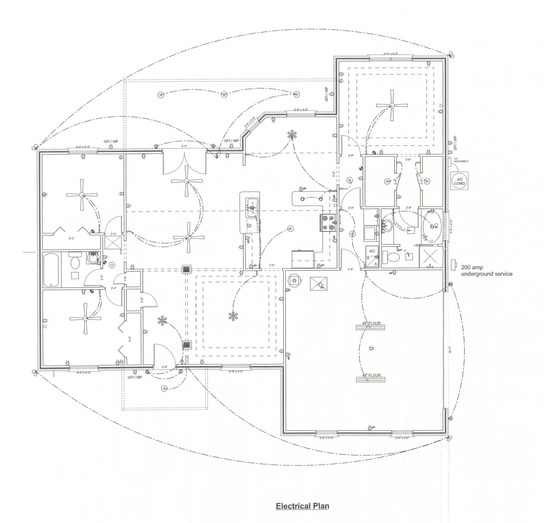
**Detail Chart** Phone Electrical panel 1--1 Wall Light SD Smoke Detector Wall light OD Flood light Chandelier 0 Globe Light Smoke Detector Floursecent Light Ceiling Fan Fan Light GFI Receptical 220 Receptical Receptical Switch Vanity light 99999 Recessed light
