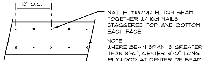
PLYWOOD FLITCH BEAM DETAIL
