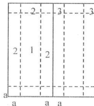
Figure 6-5 - External Pressure Coefficients, GCp Loads on Components and Cladding for Buildings w/ Ht ≤ 60 ft
