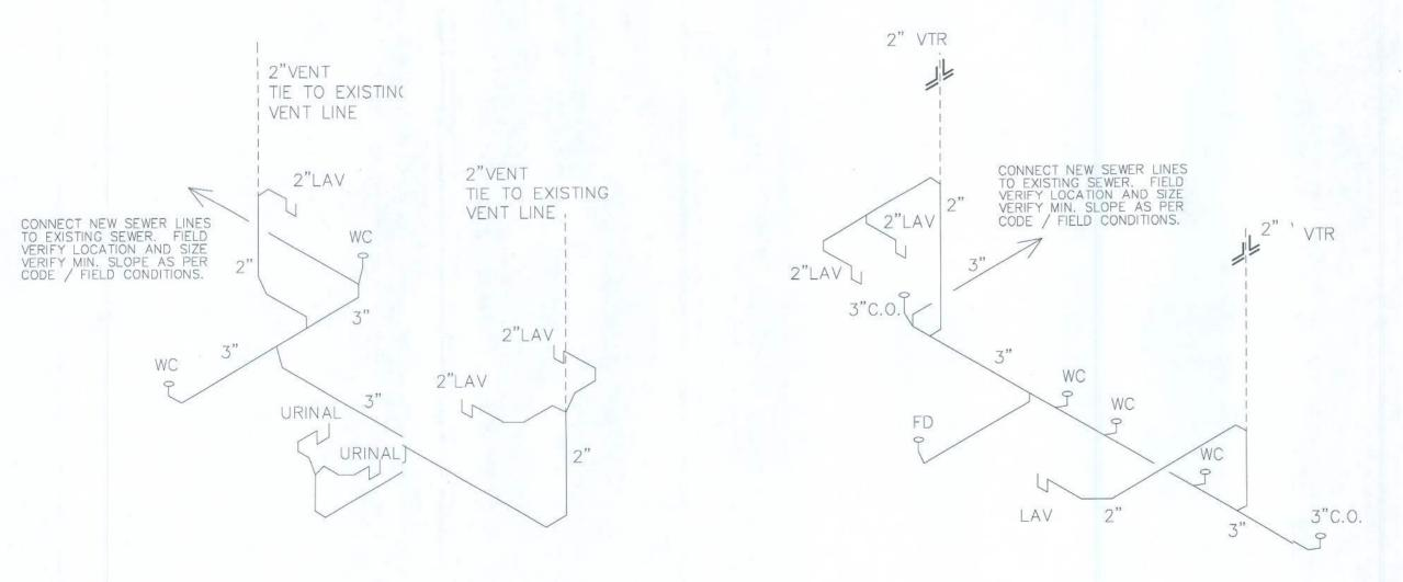
SANITARY SEWER RISER DIAGRAM
