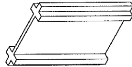
MEDIUM MULLION REINFORCEMENT #16990 ALUMINUM 6063-T6
