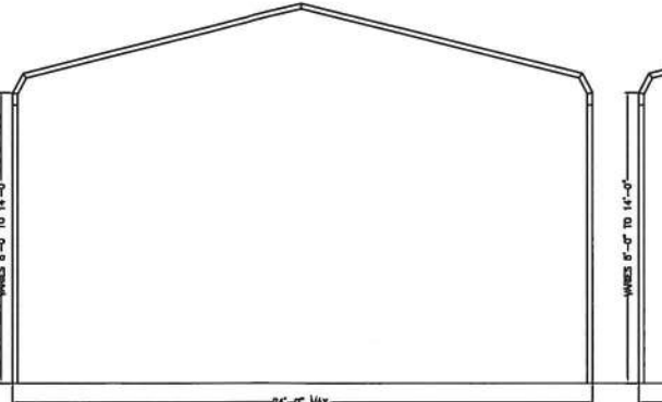
TYPICAL POST/TRUSS FRAMING SECTION - BOW FRAME, UP TO & INCLUDING 24' WIDE
