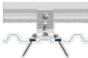
The EZ Grip Metal Deck Mount is designed to fit on the most popular R-Panel and U-Panel trapezoidal types of metal roofs. The aluminum extruded base easily clears roof profiles 7/16" tall by 1-1/2" wide. The EPDM gaskets on the washers and on the aluminum extruded base combine to provide a water tight seal at the roof penetration site.
