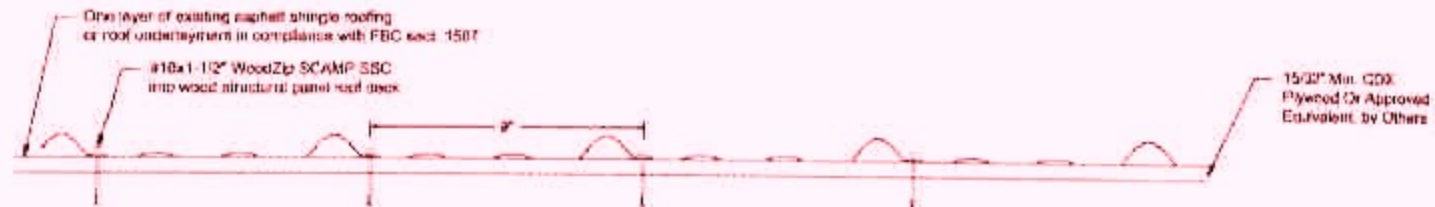
Fastener Pattern at Eave, Ridge and 3' O.C. in Field
