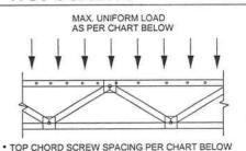
MAX. GIRDER LOAD ALONG TOP CHORD (PLF) TOP CHORD SCREW SPACING SYP or DF SPF or HF 0-4-0 1380 1050 700 0-6-0 920 552 420 0-10-0 350 1-0-0 460 344 262 1-4-0 1-6-0 306 232 276 210 1-8-0 174 2-0-0 230
