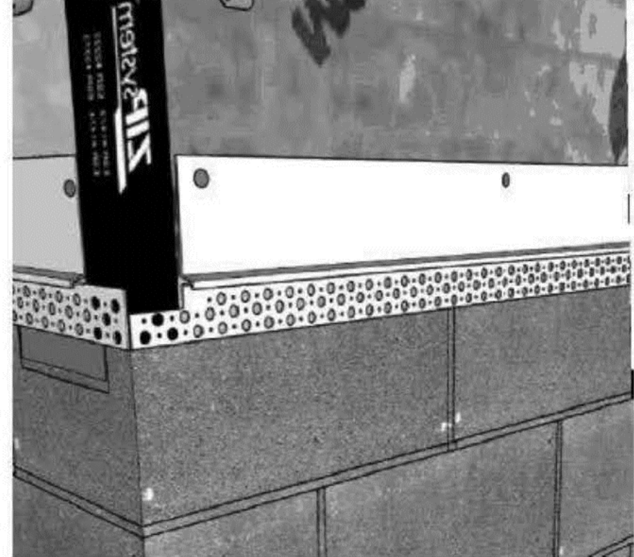
2 MID-WALL STARTER STRIP: NOTCH CORNER TO ACCEPT TRIM BEFORE INSTALLING. NOTCH TO EXTEND MIN. 3/4" BELOW TOP OF CMU
