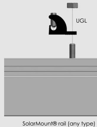
Figure 27. Slide 1/4-inch hex bolt into top mounting slot of any SolarMount® rail (standard, HD, or light). Secure nut with 7/16-inch crescent wrench with sufficient torque for lug serrations to penetrate anodized surface of rail.
