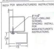
ROLL-UP DOOR TO POST CONNECTION
