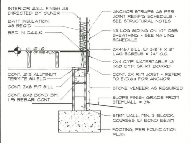
NOTE: 2X4(6) WALL STUDS SHALL BE AT 16" O.C., TYPICAL, T.O. !!
