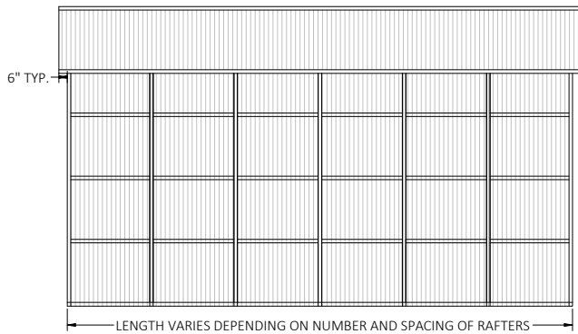
TYPICAL SIDE ELEVATION - VERTICAL ROOF/SIDING OPTION
