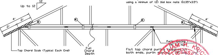
Note: If purlins or sheathing are not specified on the flat top of the sage truss, purlins must be installed at 24" o.c. max. and use Detail A.
