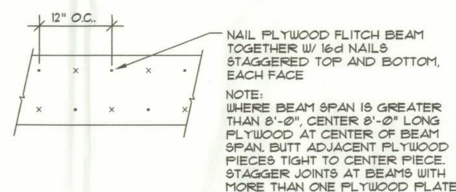
Plywood Fitch Beam DETAIL NOT TO SCALE
