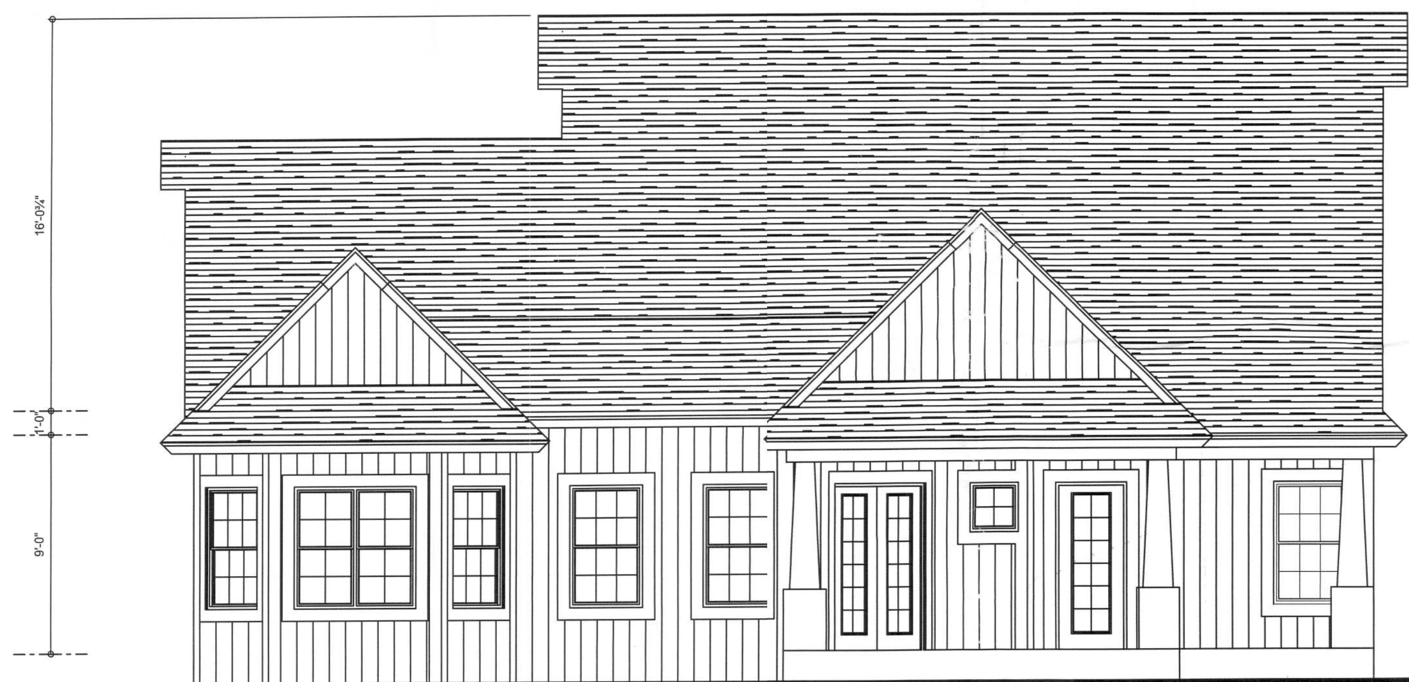
REAR ELEVATION SCALE: 1/4" = 1'-0"
