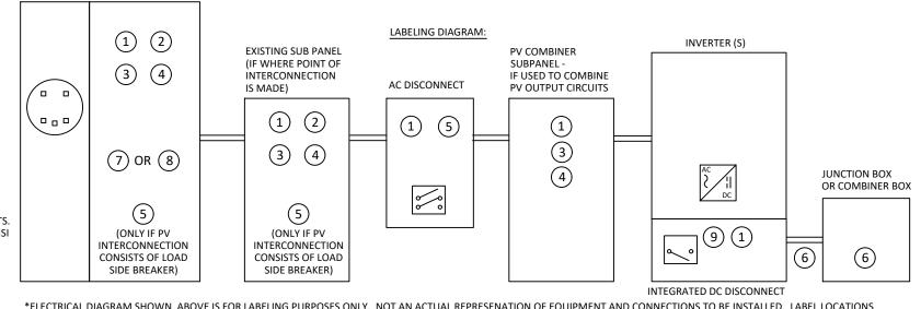
\*ELECTRICAL DIAGRAM SHOWN ABOVE IS FOR LABELING PURPOSES ONLY. NOT AN ACTUAL REPRESENATION OF EQUIPMENT AND CONNECTIONS TO BE INSTALLED. LABEL LOCATIONS PRESENTED MAY VERY DEPENDING ON TYPE OF INTERCONNECTION METHOD AND LOCATION PRESENTED ON THE ELECTRICAL DIAGRAM PAGE.
