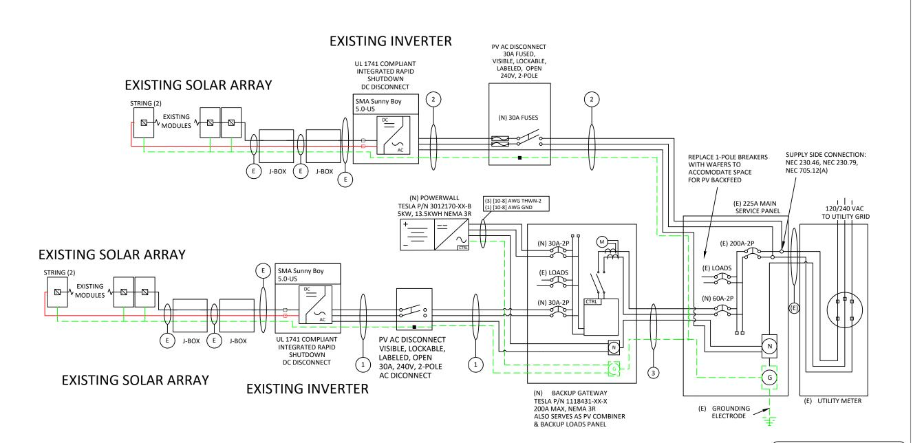
VISIBLE, LOCKABLE, LABELED AC DISCONNECT **LOCATED WITHIN 10'** OF UTILITY METER
