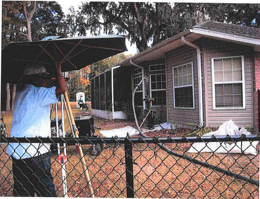
Level to monitor structure movement
