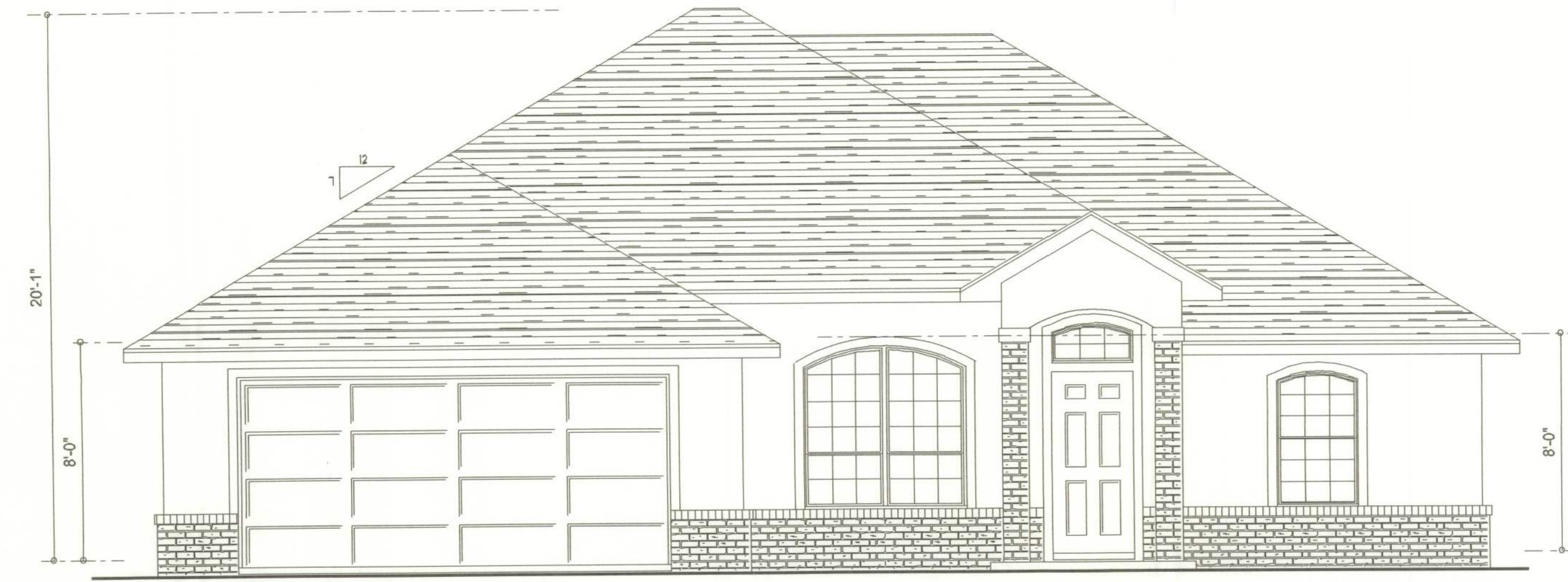
FRONT ELEVATION SCALE: 1/4" = 1'-0"
