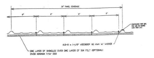
MINIMUM 29 GA. ULTRA-RIB PANEL TYPE #2 FASTENER PATTERN AT 12" O.C.
