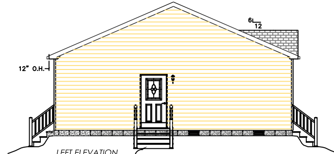
LEFT ELEVATION HANDICAP RAMP(S), STAIRS(S), AND HANDRAILS ARE SITE INSTALLED, DESIGNED BY OTHERS, AND SUBJECT TO LOCAL JURISDICTION.
