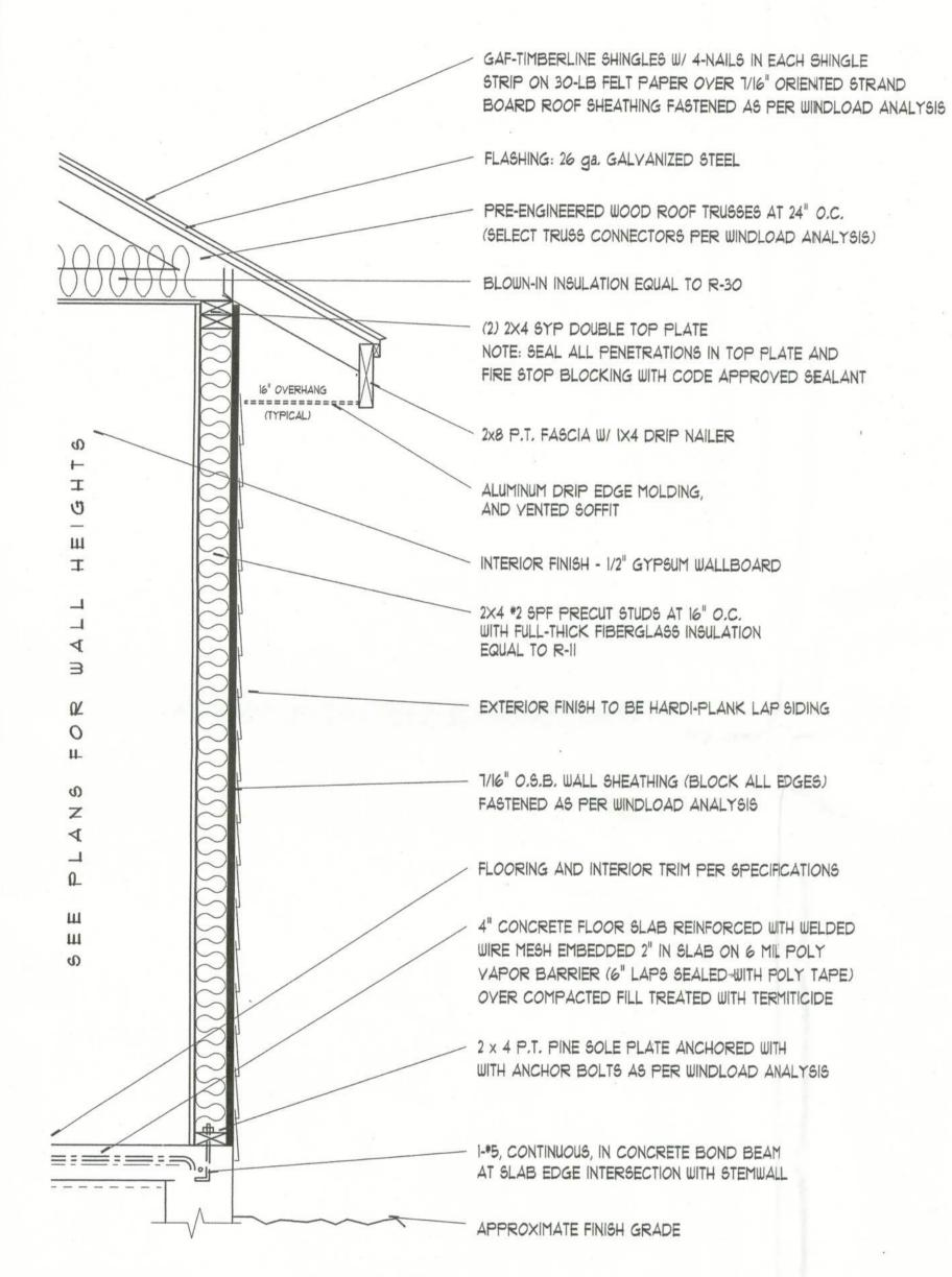
TYPICAL WALL SECTION SCALE: 1" = 1'0"
