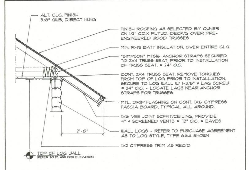
Truss Anchor DETAIL
