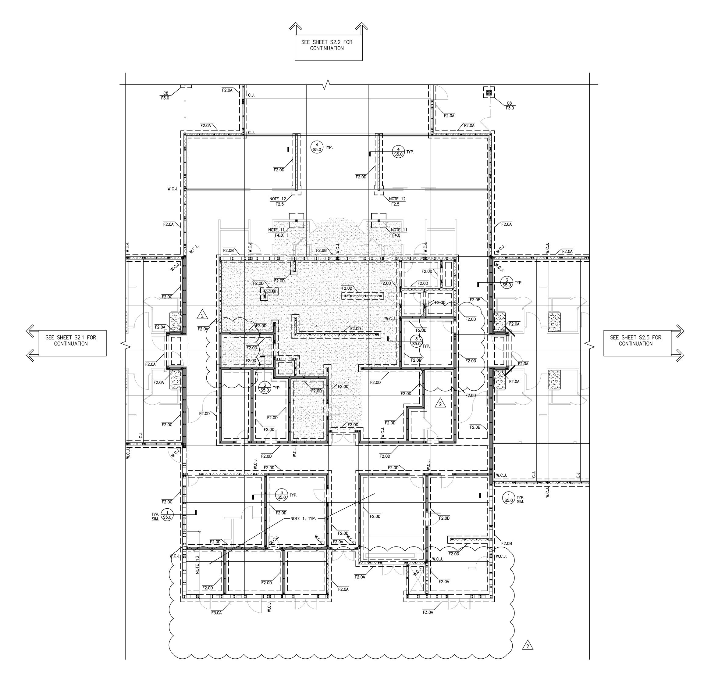
FOUNDATION PLAN NOTES: I. 4" CONCRETE SLAB ON GRADE W/ (1) LAYER OF 6x6 W1.4xW1.4 W.W.F. REINF. OR FIBERMESH REINF. ON 15 MIL VAPOR BARRIER ON PREPARED 2. CL TYPICALLY DENOTES CONTROL JOINT PER DETAIL ON \$4.0.
