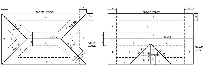
ROOF SHEATHING NAILING ZONES (HIP ROOF)
