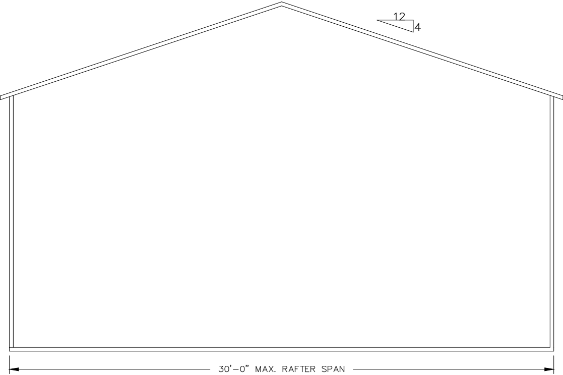
TYPICAL BOX EAVE RAFTER END WALL FRAMING SCALE: NTS
