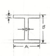
I-BEAM SHOWN NOT TO SCALE DIMENSION IN TABLE ARE ACTUAL. DIMENSION FROM AMERICAN STANDARD BEAMS
