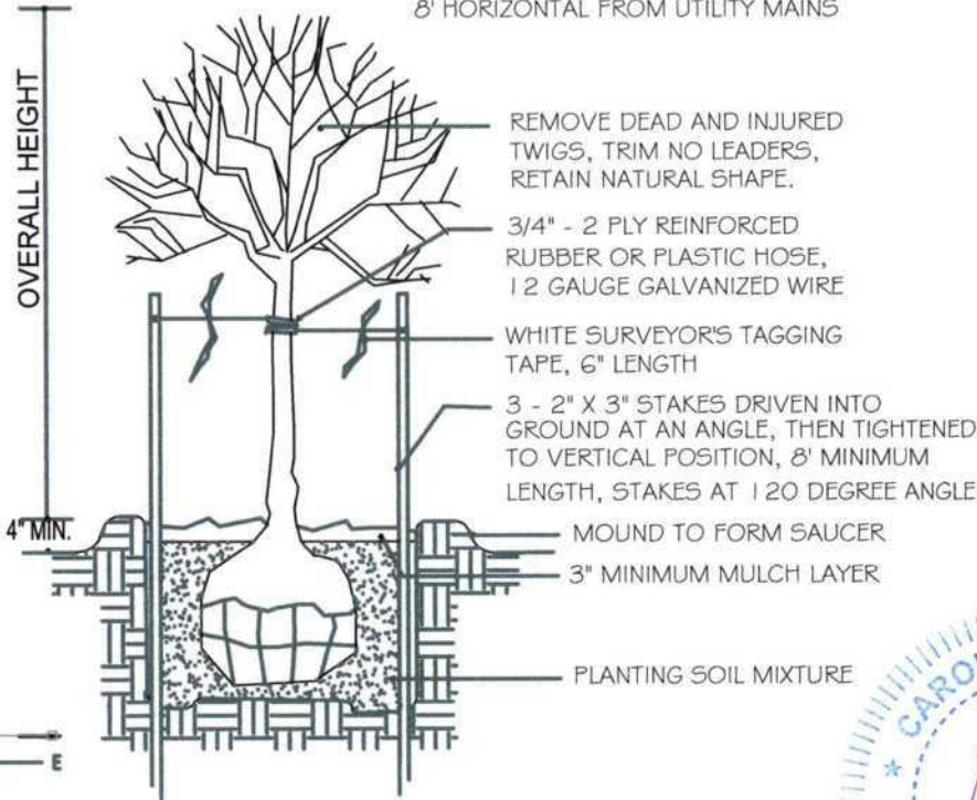
TREE STAKING AND PLANTING DETAIL
