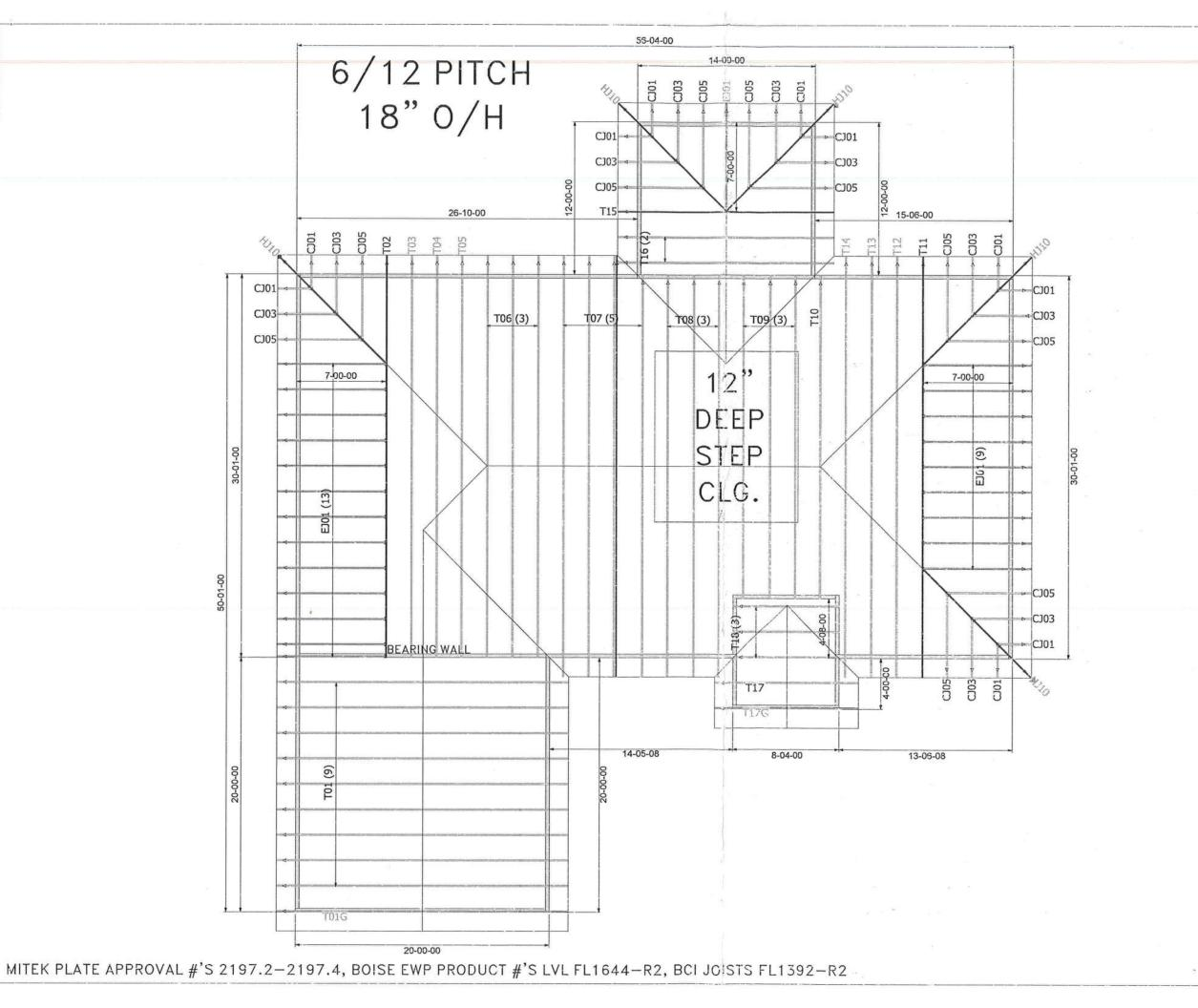
THE ARROW HEAD AT THE END OF THE TRUSS ON THE TRUSS PLACEMENT CORRESPONDS WITH THE LEFT SIDE OF THE INDIVIDUAL TRUSS DRAWING, USE THIS AS AN DRIENTATION GUIDE WHEN SETTING THE TRUSSES ON THE STRUCTURE.
