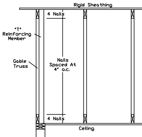
This detail to be used with the appropriate Alpine gable detail for ASCE wind load.
