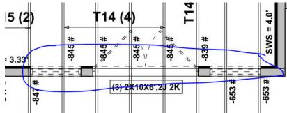
a. || || || || || || || || || || At this location run the header continuous over the two side windows with (3) kings & (2) Jacks each end & (2) jacks mid points. Also box out the header with (2) 2x6 (1) top & (1) bottom of header. Also add HTT4 hold down bottom each end & (2) MSTA24 top each end.
