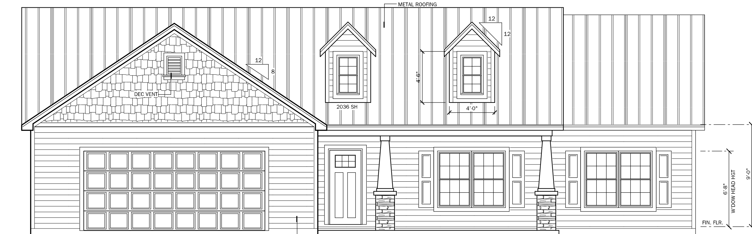
FRONT ELEVATION SCALE: 3/16" = 1'-0"
