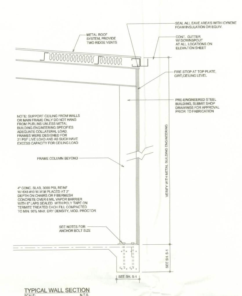
NOTE: THIS FOUNDATION DESIGN MEETS ALL REQUIREMENTS FOR WIND LOAD'S PER SBC-01, SECTION 1606, 110MPH BASIC WIND SPEED, EXPOSURE B, 1.0 USE FACTOR; BASED ON COLUMN REACTIONS IN MESCO BUILDING SEALED ENGINEERING FOR PROJECT 21-1398, DATED 11/07/03. COLUMN PAD LOCATIONS ARE TYPICAL, EXACT ANCHOR BOLT LOCATIONS AND SIZES ARE PER METAL BUILDING SEALED ENGINEERING ANCHOR BOLT PLAN.
