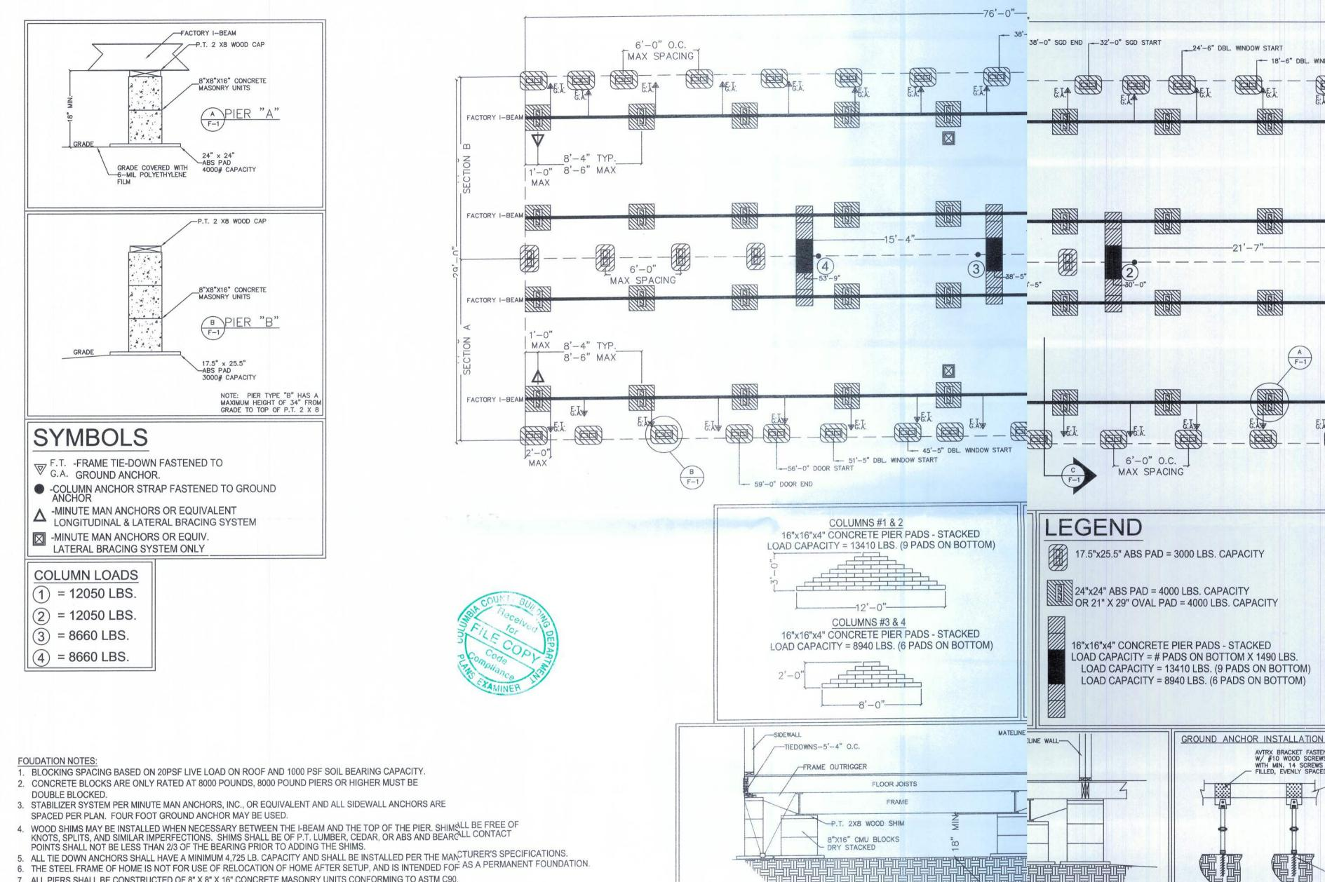
7. ALL PIERS SHALL BE CONSTRUCTED OF 8" X 8" X 16" CONCRETE MASONRY UNITS CONFORMING TO ASTM C90.
