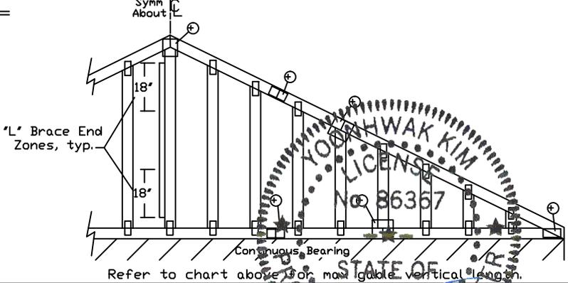
Attach 'L' braces with 10d (0.128"x3.0" min) nails.
