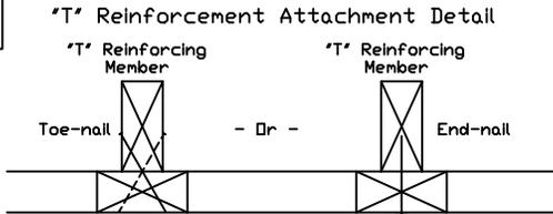
Provide connections for uplift specified on the engineered truss design.
