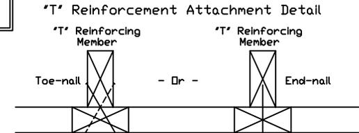
Provide connections for uplift specified on the engineered truss design.
