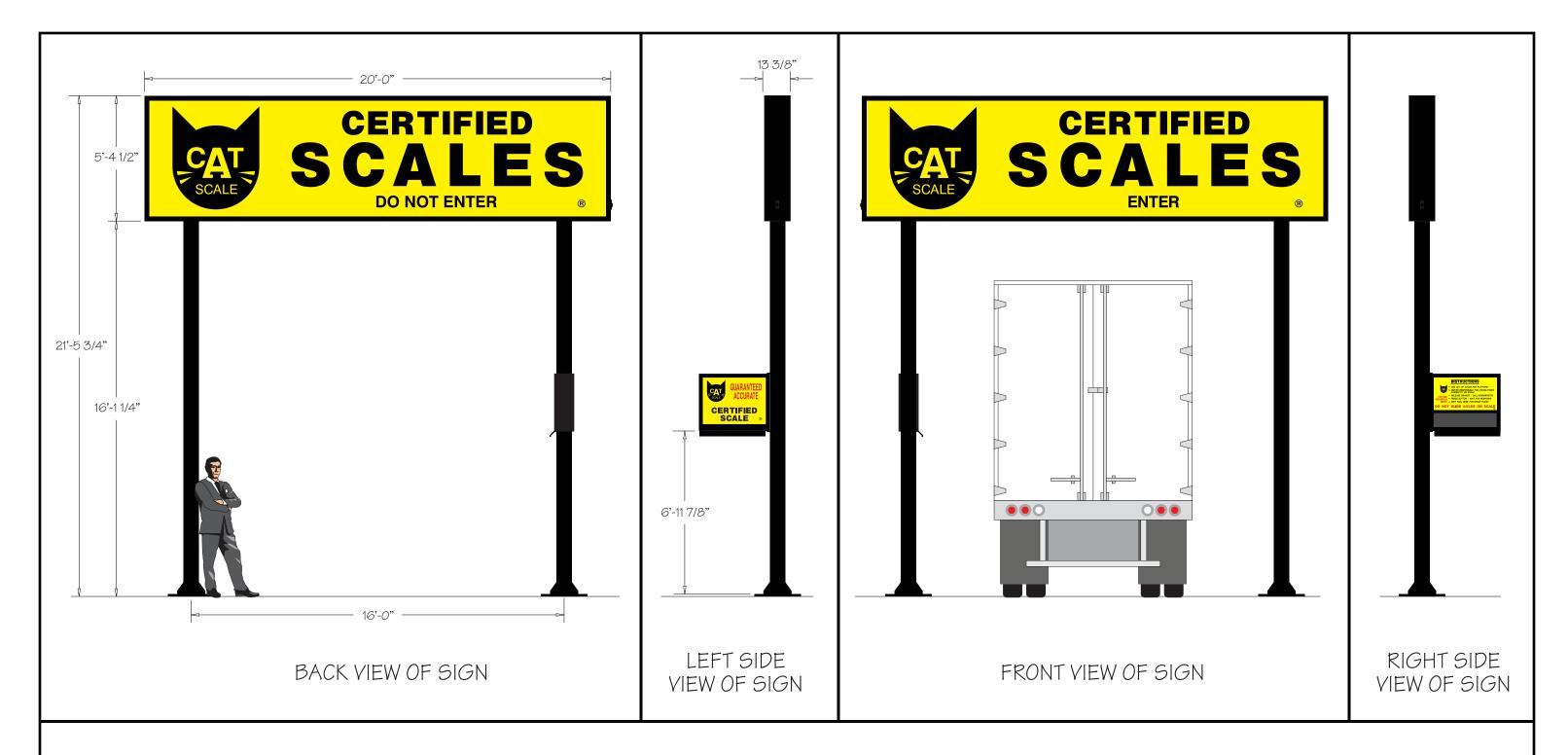
CAT Scale ID sign – Qty (7) HanleyH100W – PPS524V power supplies and Qty (20) 60" Hanley HLB-2560 Concorde 4500 LEDs. Power Consumption: approx. 490W. Speaker Sign – (1) Qty (1) HanleyH100W – PPS524V power supply and Qty (3) 36" Hanley HLB-2560 Concorde 4500 LEDs. Power Consumption: approx. 49W.
