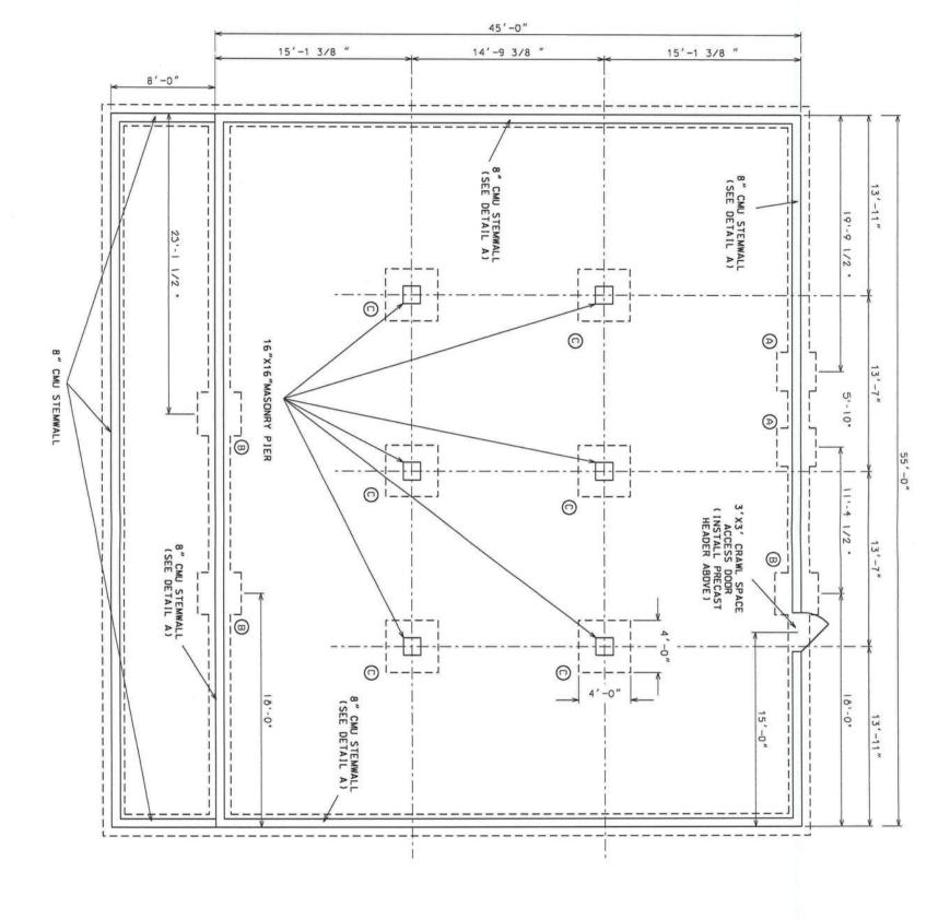
3.) Footer "C" shall be 14" thick with one reinf. mat of 7-#5 rebars each way. (3000 psi conc.)
