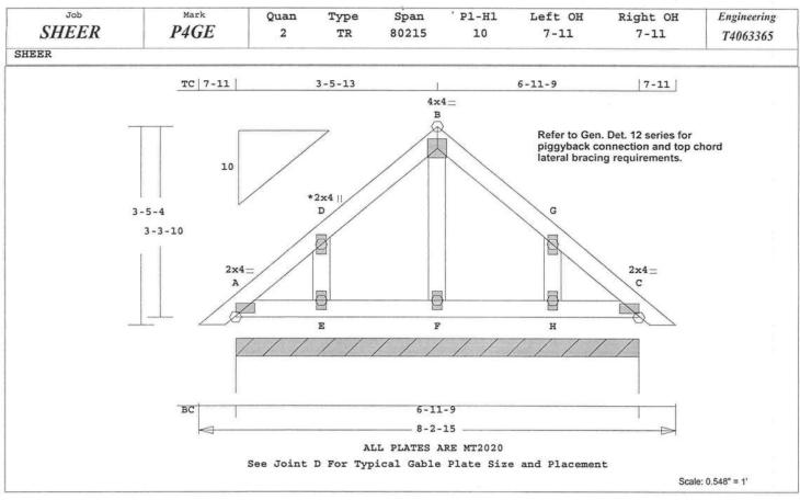
Online Plus -- Version 28.0.007 RUN DATE: 27-APR-11 CSI -Size- ----Lumber----TC 0.02 2x 4 SP-#2 0.02 2x 4 SP-#2 BC 0.01 2x 4 SP-#2 Brace truss as follows: To O.C. From 0- 0- 0 8- 2-15 TC Cont. Cont. 0- 0- 0 8- 2-15 psf-Ld Dead Live TC 10.0 20.0 BC 10.0 0.0 TC+BC 20.0 20.0 40.0 Spacing 24.0" Total Lumber Duration Factor 1.25 Plate Duration Factor 1.25 TC Fb=1.15 Fc=1.10 Ft=1.10 BC Fb=1.10 Fc=1.10 Ft=1.10 Total Load Reactions (Lbs) Jt Down Uplift Horiz-559 78 U 60 R
