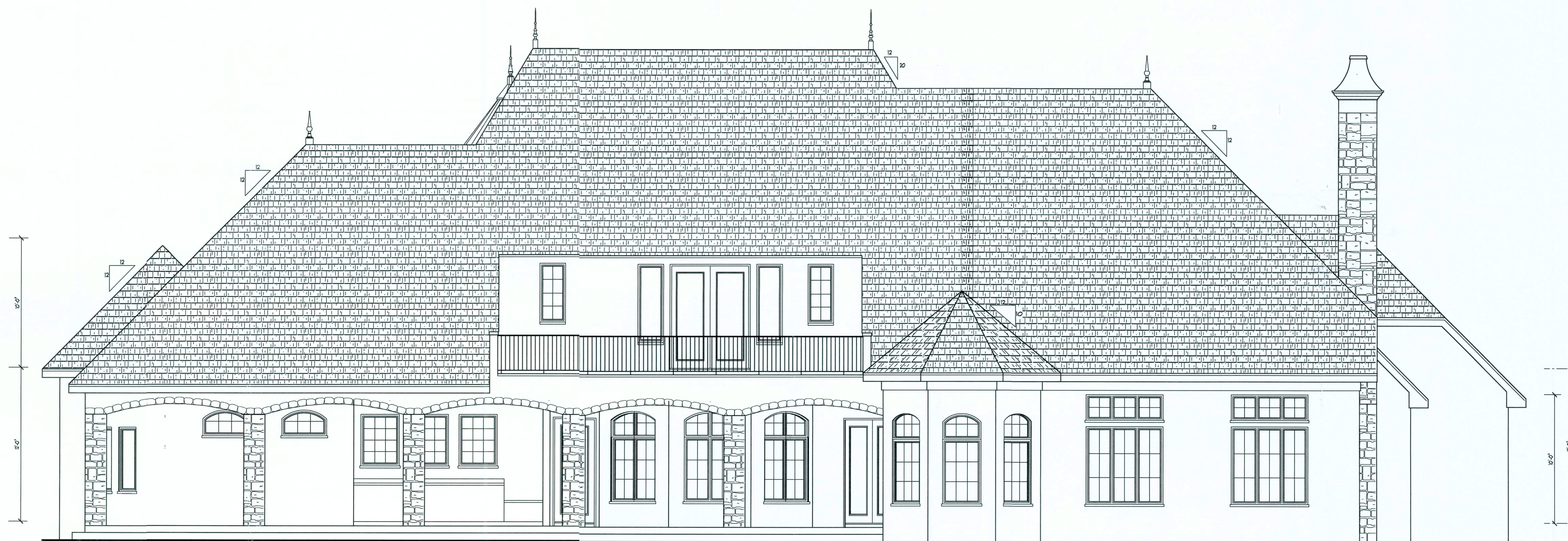
REAR ELEVATION SCALE: 1/4" = 1'
