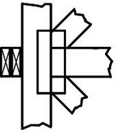
Indicates location where bearings (supports) occur. Icons vary but reaction section indicates joint number where bearings occur. Min size shown is for crushing only.
