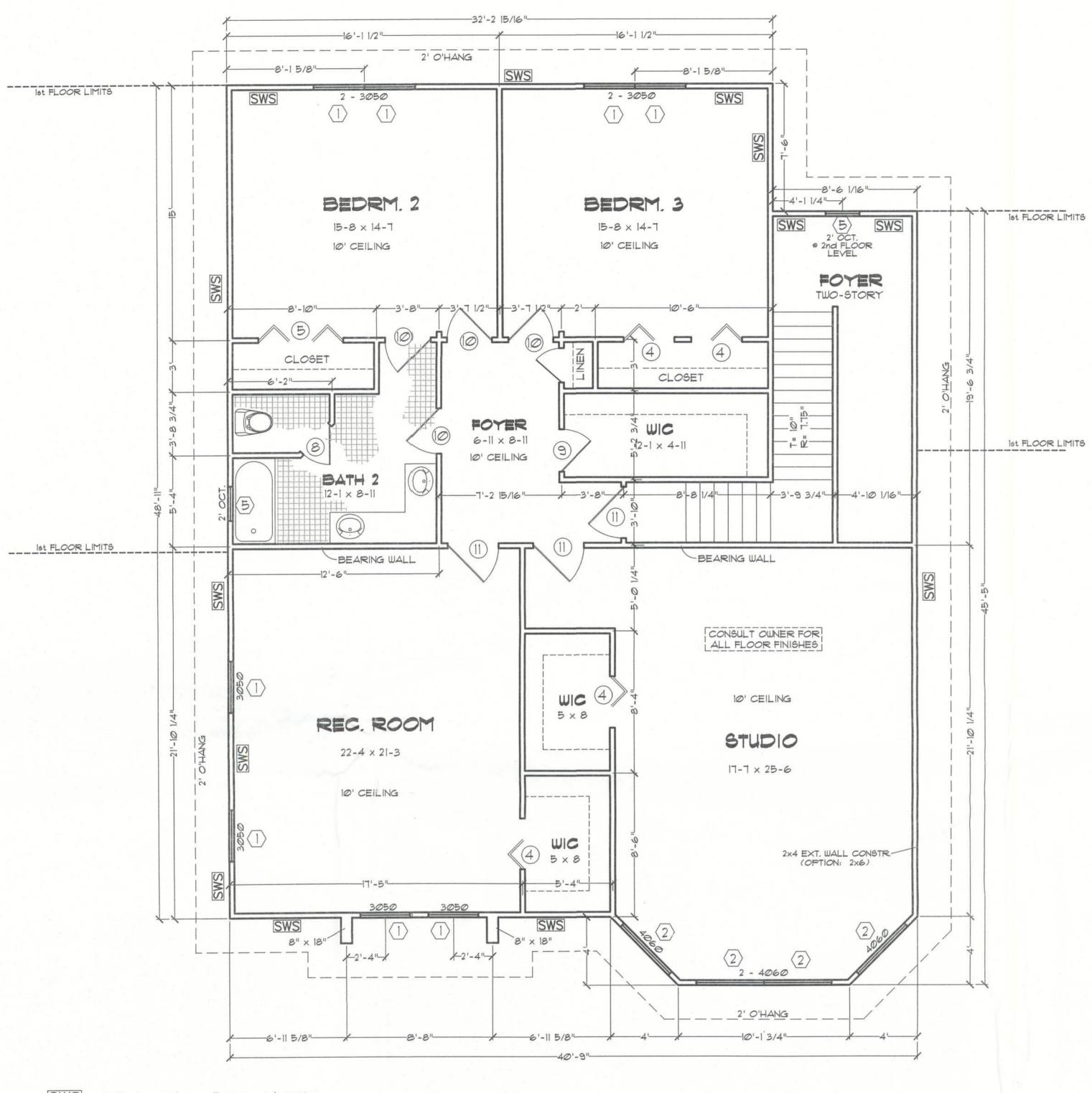
SWS = Indicates a shearwall segment location referring to the labeled section of wall lying between the adjacent window / door openings in either direction. The shearwall areas have a height/width aspect ratio of 3-1/2: I or wider.
