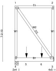
LOADING (psf) SPACING-**GRIP** CSI. DEFL. **PLATES** 2-0-0 (loc) I/defl L/d Plate Grip DOL TCLL 20.0 1.25 TC 0.48 Vert(LL) 0.05 3-4 >999 240 MT20 244/190 BC **TCDL** 10.0 Lumber DOL 1.25 0.63 Vert(CT) -0.08 3-4 >737 180 **BCLL** 0.0 Rep Stress Incr NO WB 0.00 Horz(CT) 0.00 n/a n/a Code FBC2023/TPI2014 Weight: 51 lb FT = 20%**BCDL** 10.0 Matrix-MP
