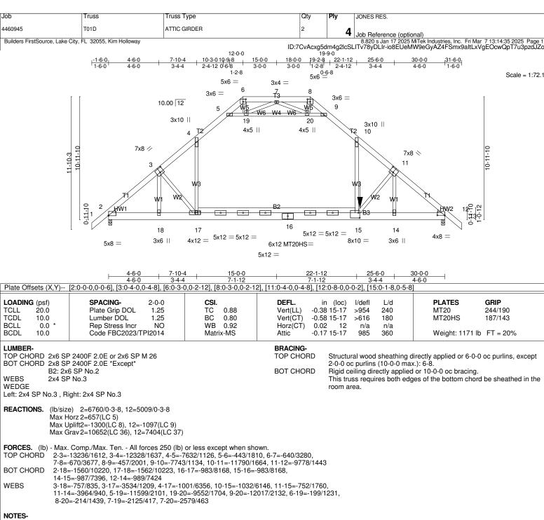
1) 4-ply truss to be connected together with 10d (0.131"x3") nails as follows:
